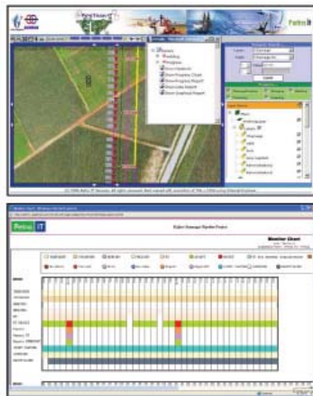
Geo-enabling daily activity allows a direct correlation between progress "March Charts" and map display
